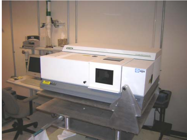
Figure 6. Digilab FTS6000 Fourier Transform Spectrometer
