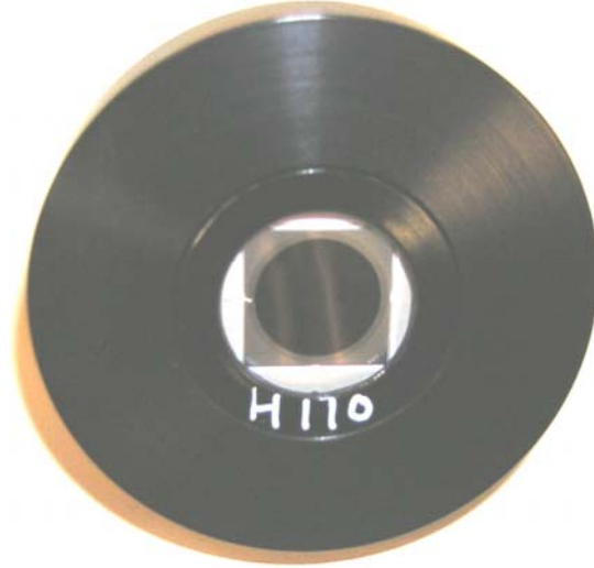
Figure 9. UV-Visible Spectral Reference Detector
